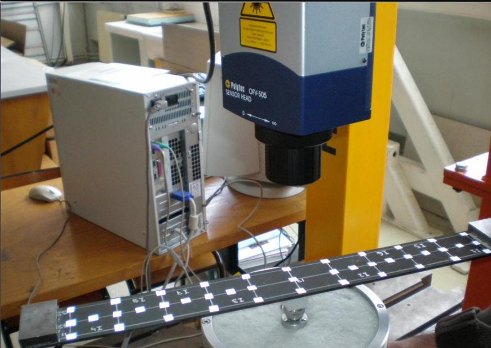
Vibration test based on Oberst Beam method
