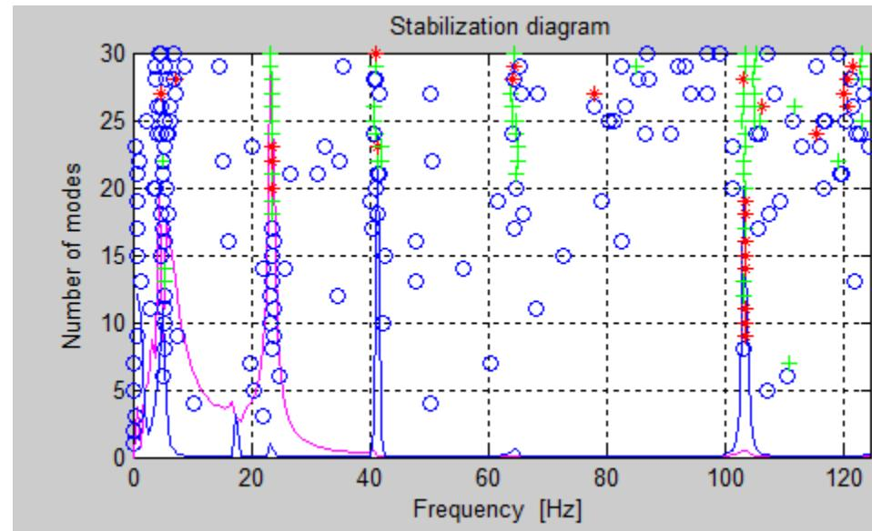
Stabilization criteria : Frequency = 2% , Damping = 5%
