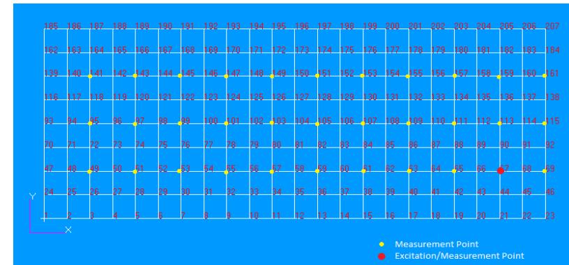
Plate clamped at one side excited so to extract torsional and bending modes
