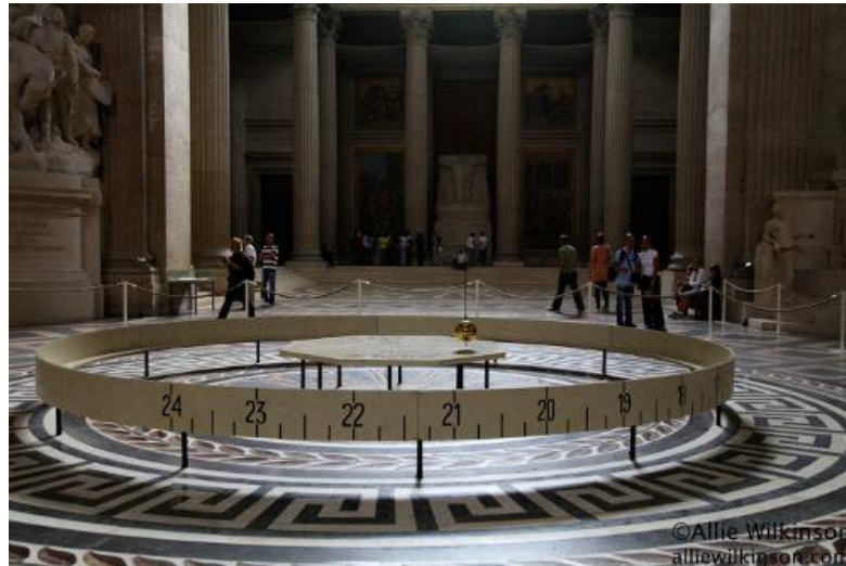
Figure 4: The Foucault pendulum at the Panthéon of Paris, France, used to show the Earth rotates on its axes. It has a nonlinear behavior for big amplitudes.
