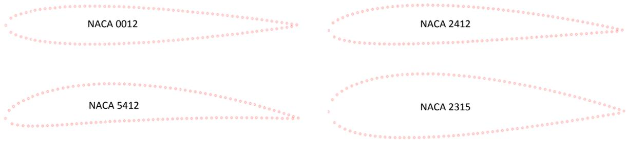
**Figure 6 - Examples of NACA 4-Digits Series automatically generated in Patran.**
