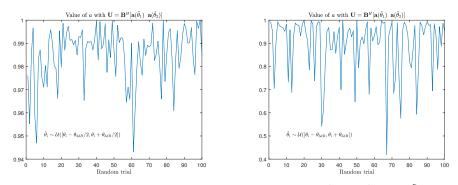
Case of 2 interferences located at  $\theta_1, \theta_2$ . Value of a when  $\mathbf{U} = \mathbf{B}^H \begin{bmatrix} \mathbf{a}(\tilde{\theta}_1) & \mathbf{a}(\tilde{\theta}_2) \end{bmatrix}$  and  $\tilde{\theta}_i$  drawn randomly around  $\theta_i$ .
